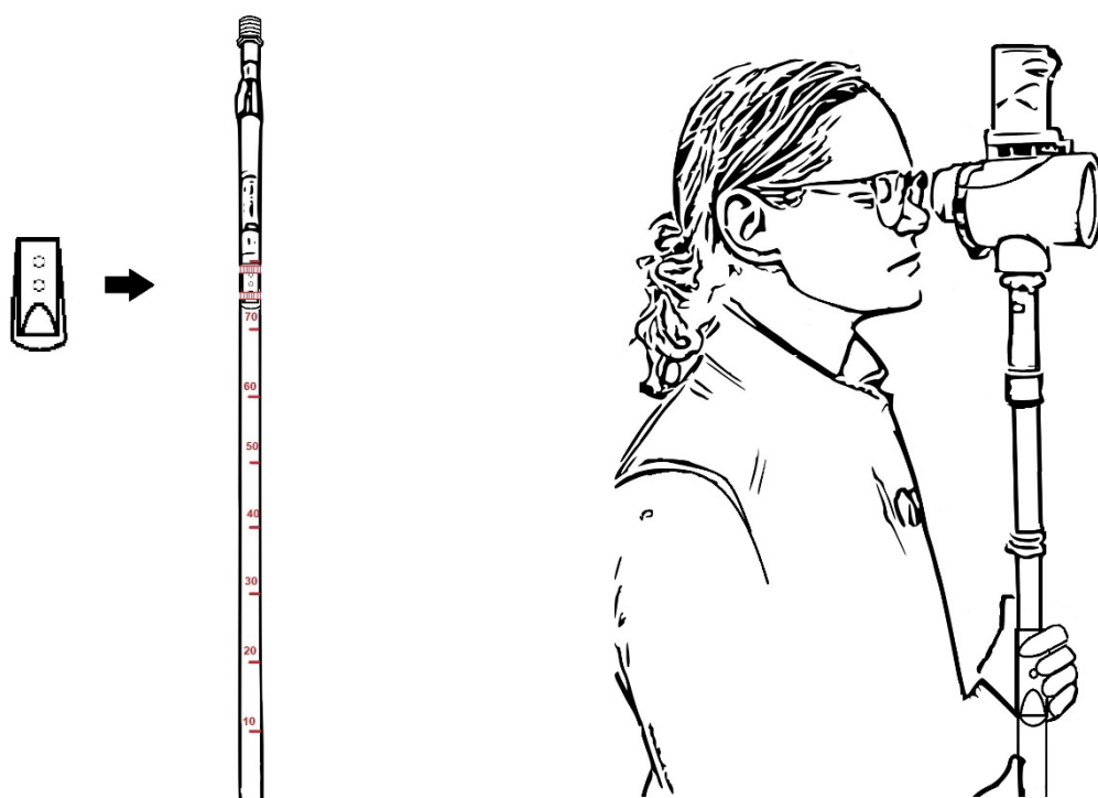
Figure 8. the laser pointer attached at a point comfortable for the observer to use without changing position when looking through the densitometer
