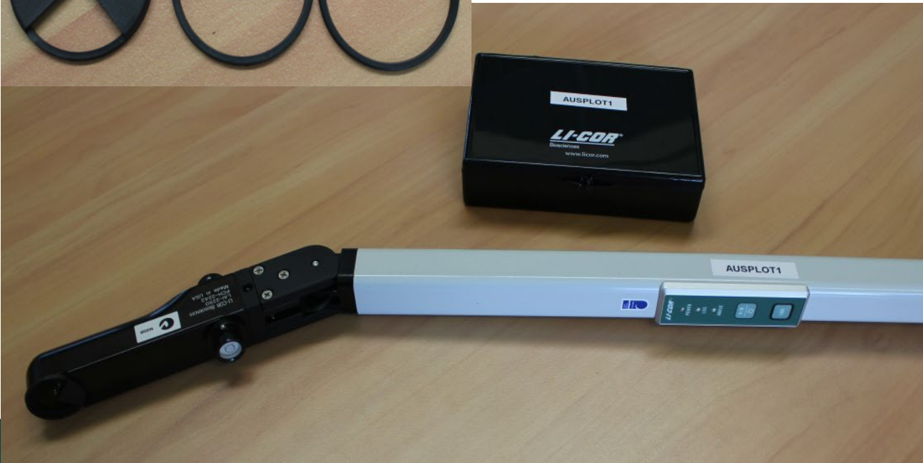
The Sensor head and fitting the lens cover
